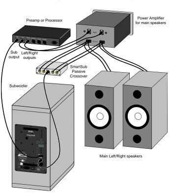
The SmartSub Integrator in augment configuration should be used if a passive crossover is not available for your main speakers, you desire adjustability of the main channel bass level or extension, or if you desire more than one subwoofer in your system, or two stereo subwoofers.
